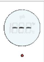
This indicates an invalid reading. This is due to incorrect usage, such as:
