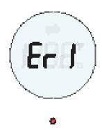
An Error message indicates an internal problem with the thermometer.
