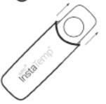
2 Grab the ARC InstaTemp on its sides and pull out of the case.
