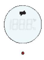
Steady battery symbol & red indicator light: insufficient battery power for a measurement. Refer to page 23, Warranty
