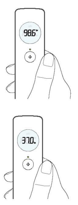
Press and release the activation button to get a reading. Once the reading appears on screen in Fahrenheit, press and release the activation button again —the reading will automatically change to Celsius. Repeat to change back.
